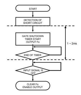
(1)In case the gate signal is "ON" and the collector voltage is high, the gate driver will recognize the circuit as short circuit and immediately reduce the gate voltage.(Soft shut down) Besides, put out an Fo sign which inform that protection circuit is operating.
